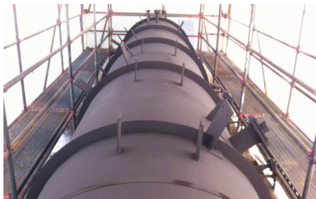
Image: PPG Hi-Temp 1027 can be applied on hot substrates as well as on substrates which serve in conditions with severe thermal shocks to cryogenic temperature exposure.
