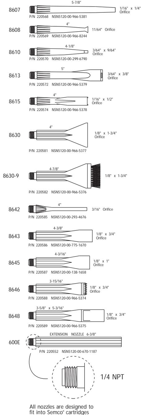
All nozzles are designed to fit into Semco® cartridges
