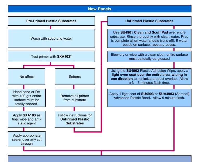
Continue with the repair using your preferred PPG or *Nexa Autocolor* paint system undercoats and topcoats. Please refer to the product data sheet of the product that will be applied next for further information on how to best properly complete your repair
