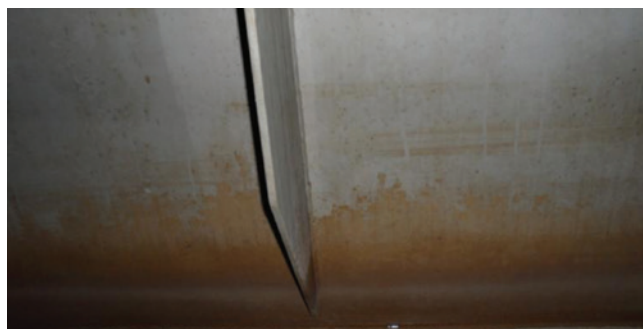
Images: After 5 years of extensive use, the water ballast tanks of the Kristin C are in excellent condition as a result of the outstanding anti-corrosive properties of the SIGMACOVER 380 coating
