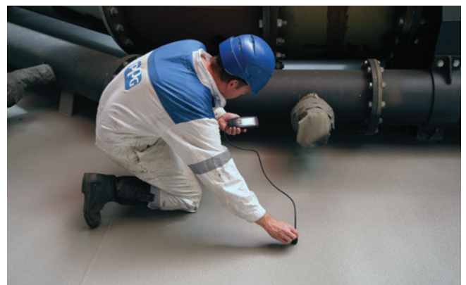
Images: Measuring the thickness of the SIGMASHIELD system
