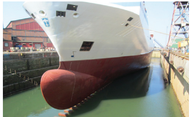
Image: After two winters operating in heavy ice conditions the underwater hull of the SEAGARD is still in perfect condition.
