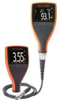
Figure 6: Electromagnetic depth gauge
