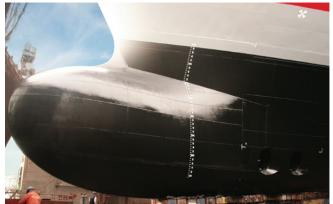
Image: The SIGMASHIELD 1200 coating after application on the Bothniaborg
