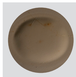
Failed After 14 days at 70°C/158°F with other phenolic epoxy tanklining.
