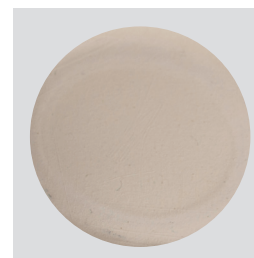
Pass After 14 days at 70°C/158°F with PPG PHENGUARD 985.
