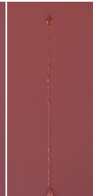
The release effect of CSPs creating a slippery surface and low friction properties
